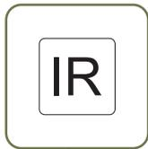
Stick the receiver of an external IR cable to this location when the cable is not used or the product is moved.
